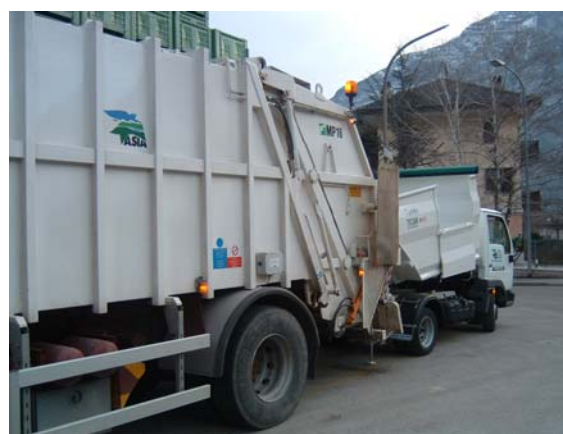
Image 2: Unloading of food collection vehicle into RCV for onward haulage - Northern Italy
