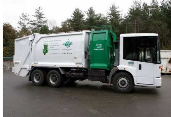
Image R: Split bodied vehicle used in the Isle of Wight for combined food and garden waste collections
