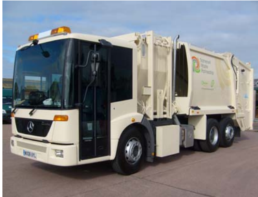
Image Q: 3 way split vehicle tested in Somerset with pod for food waste and compaction chambers for plastic and cardboard
